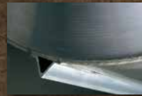
Heavy-Duty V-Keel Ensures even tracking in the water while protecting the bottom of pontoons.
